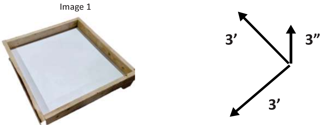
Image 1 shows the inside of the test box each formula was injected into under confinement.
